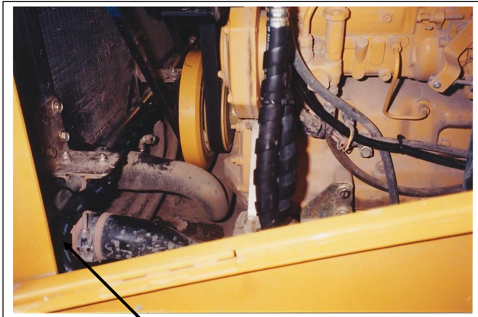
13/32" hose running across the bottom of the radiator towards the condenser fitting on the left side of the radiator
