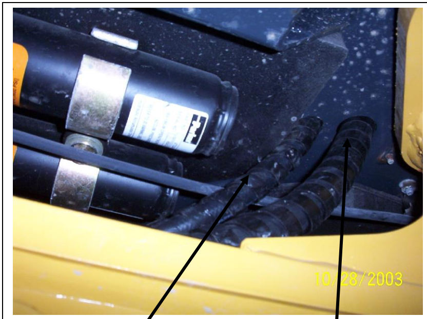
5/16" line going up into the cab.
